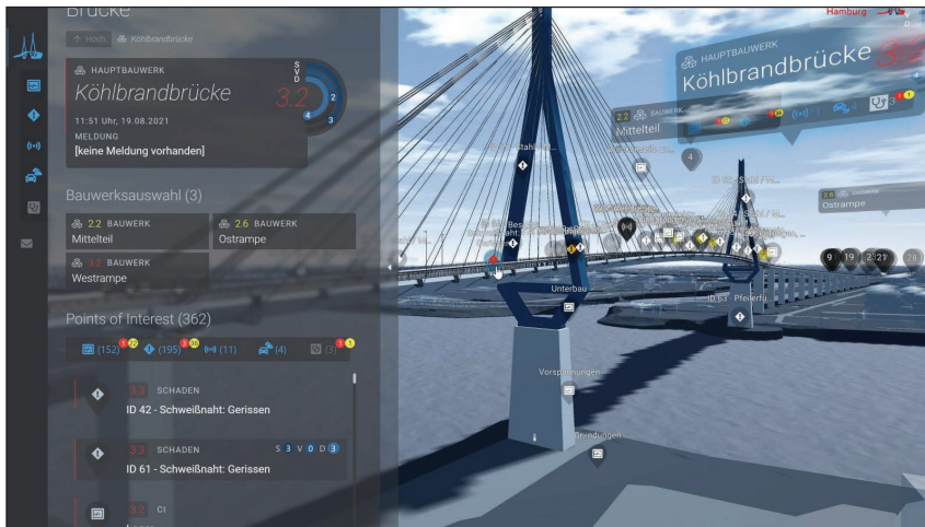
FIGURE 4 – A visualization of the digital twin of the Köhlbrandbrücke. (Source: copyright SMART-bridge Hamburg, taken from [29].)
