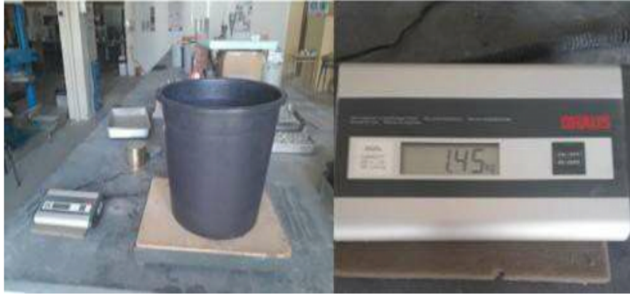
Figure 3.5: Mass of container with water.
