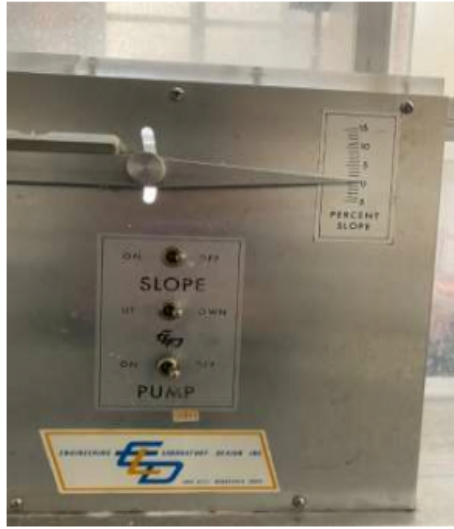
Figure 3.6: The configuration of the water tunnel and the slope that defines the velocity.[18]
