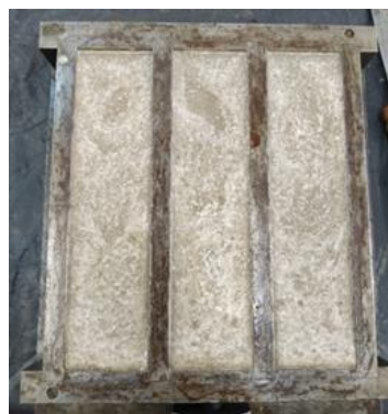
Mould design for producing mortar specimens.
