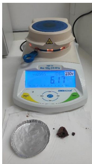
Figure 9. Equipment used to determine moisture content.
