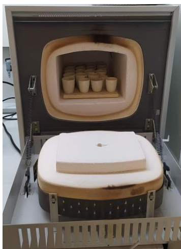
Figure 10. Muffle with crucibles inside.
