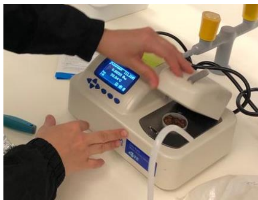
Figure 21. Measurement of aw using the AquaLab S4TE equipment.
