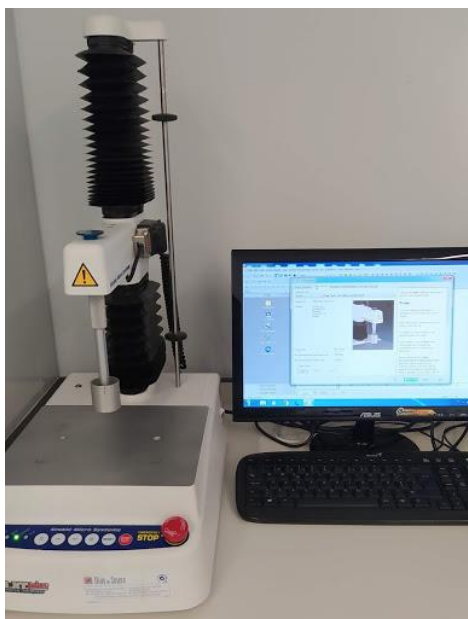
Figure 23. Texturometer with 30 kg load cell and cylindrical P/35 aluminum probe.
