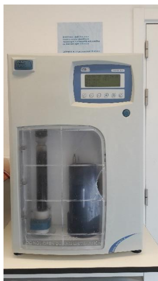
Figure 11. Kjeldahl distiller used for protein content analysis.
