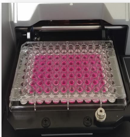
Figure 17. Microplate used in the determination of cytotoxic activity.
