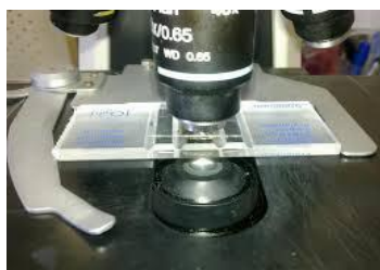
Figure 15. Equipment used for fluorescence measurement to quantify cellular antioxidant activity.
