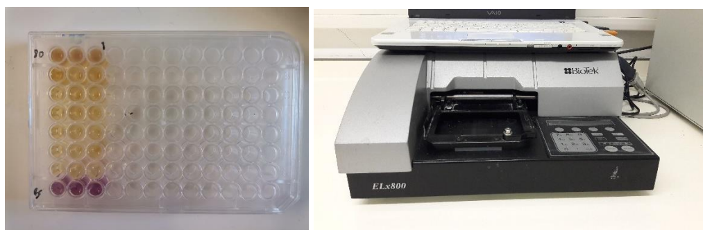
Figure 13. Plate and equipment used for the measurement of absorbance by the DPPH method.
