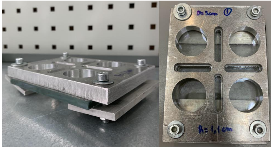
Figure 19 - Mold used to make the PDMS/Surfactant samples.
