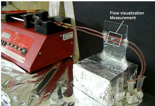
Fig. 2 Experimental setup for the dynamic sedimentation measurements.
