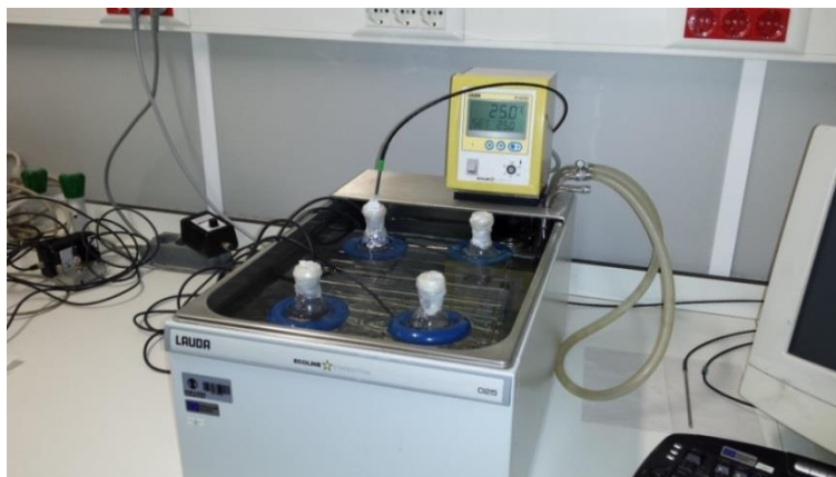
Figure 14 - Experimental setup used on the shake flask method.
