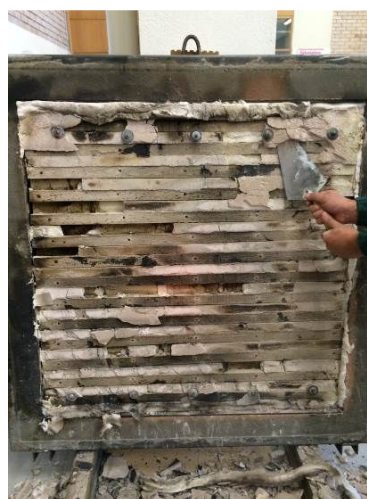
Fig. 11 - Timber structure after the test (th = 5 mm)
