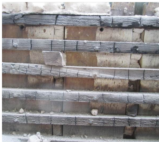
Fig. 5 - Timber structure after the test ( th = 15 mm)
