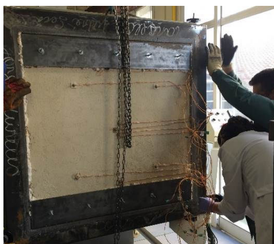
Fig. 2 - Experimental set up of tabique wall panel
