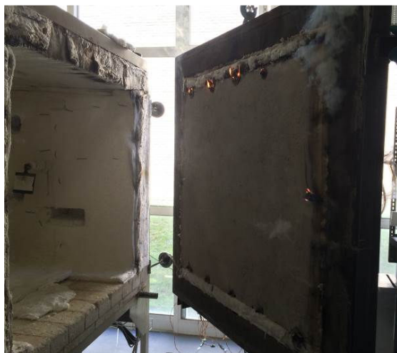
Fig. 4 - Tabique wall panel at the end of the test ( th = 15 mm)
