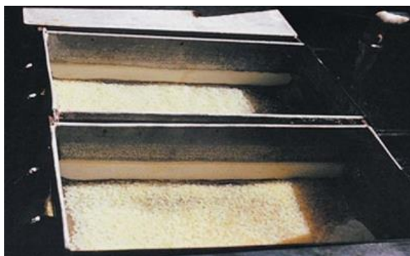
Figura 1.8. Incubadora Sandfort (adaptado de Hoitsy et al. 2012)
