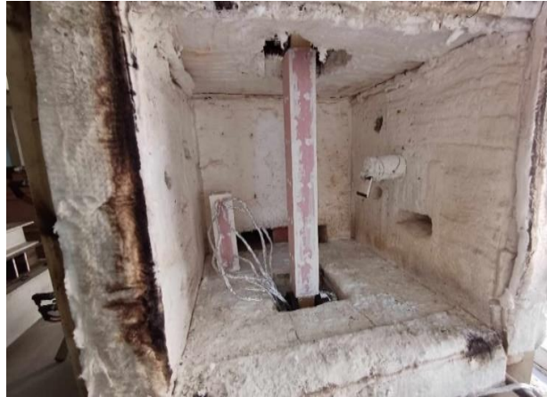
Figure 11: Preparation of the specimen inside the furnace.
