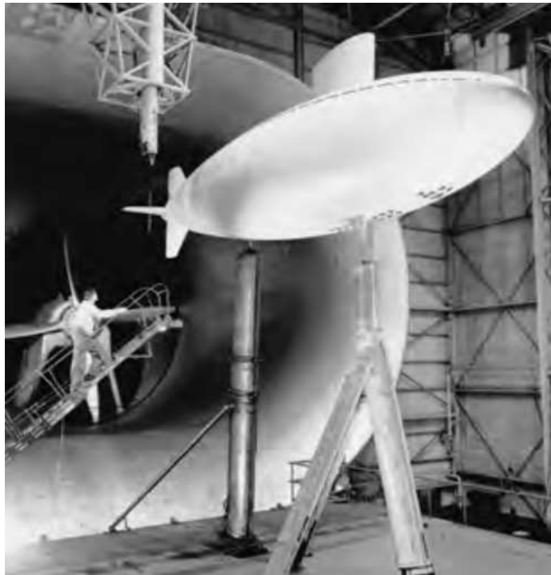
Figure 15. Submarine model in test section in the wind tunnel [2].
