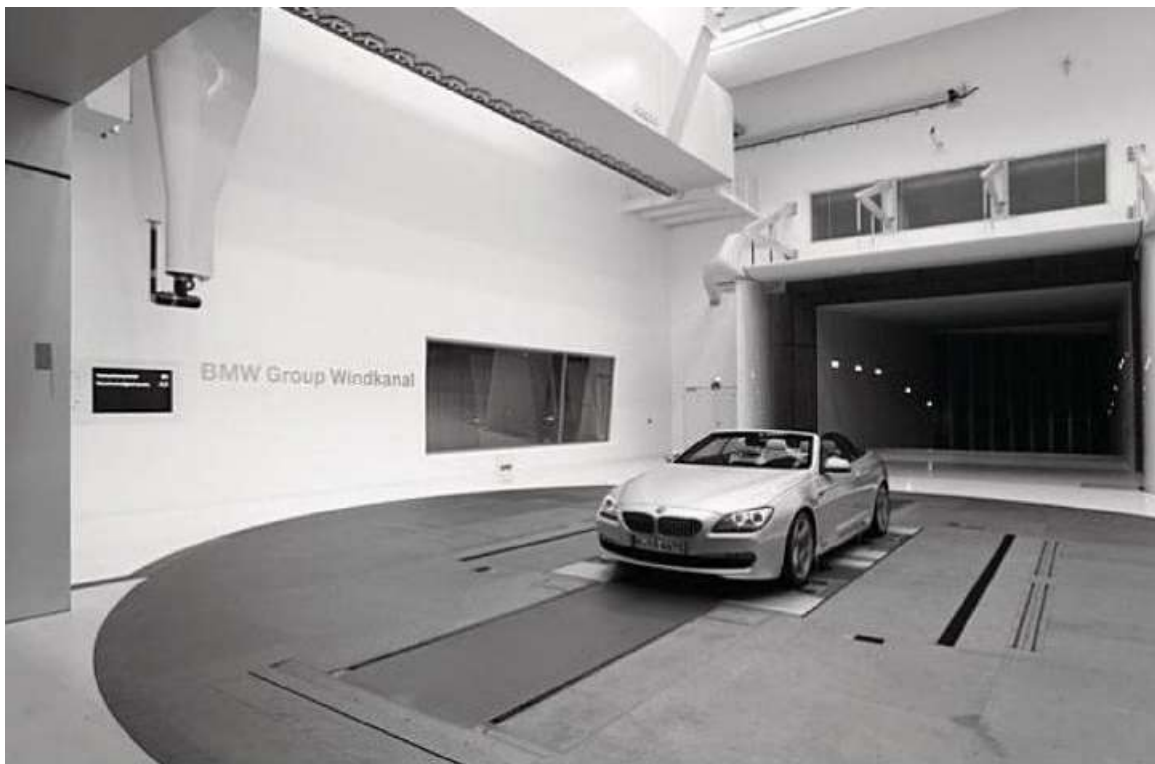
Figure 19. Car in the test section of an automotive wind tunnel at the Aerodynamic Test Center of BMW in Munich Germany [10].
