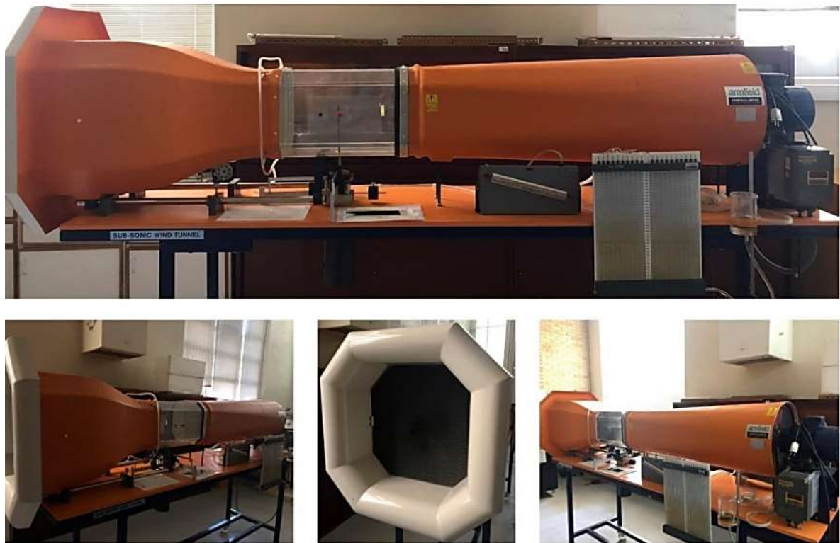
Figure 29. Open circuit subsonic Wind tunnel provided by IPB [23].
