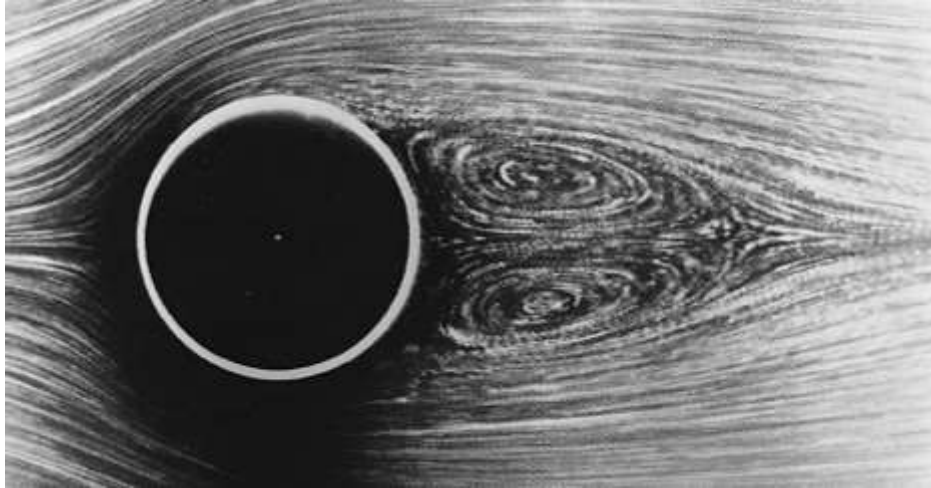
Figure 8. Laminar flow over a cylinder with Re = 26 [1].
