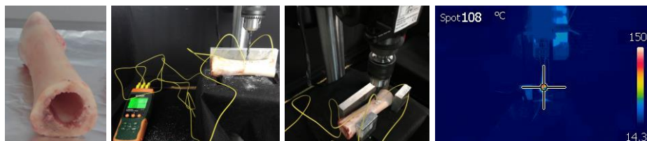
Fig. 1 – Drilling tests on cortical bone and temperature measurement system.
