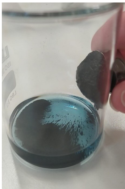
Figure 6. Metallic particles attracted by a magnet.
