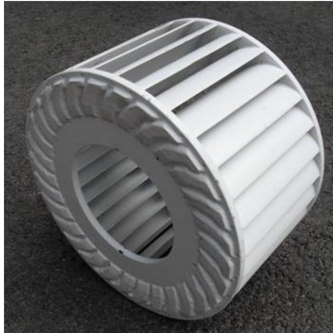
Figure 2.7: Cross-flow turbine runner [36].
