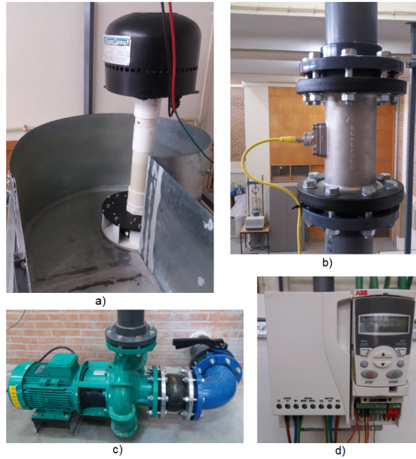
Figure 3.9: Low Head Emulation System main components. a) LH400 turbine. b) VFI 12-240 DN100 water flow sensor. c) CronoBloc-BL 125/185-5,5/4 water pump. d) ACS355-03E-12A5-4+J404 frequency converter.
