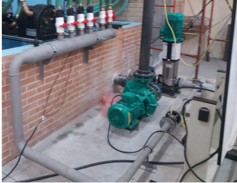
Figure 3.3: Pipeline used in the Heads Emulation System
