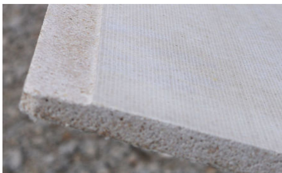
Figura 3.2 (e): Placa MgO – MAGNESIOPAN FONTE: (Magnesiopan, 2020).
