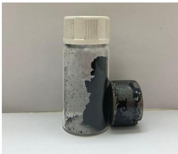
Figure 15. An example of magnetism of the synthesized CNT.
