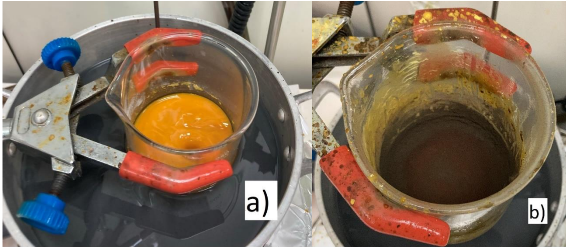
Figure 10. a) Catalyst at 60 °C. b) Catalyst at 200 °C.
