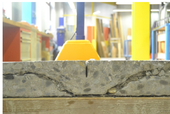
Figure 5 – Cracking pattern and internal shear crack of reference slab BC01 after failure
