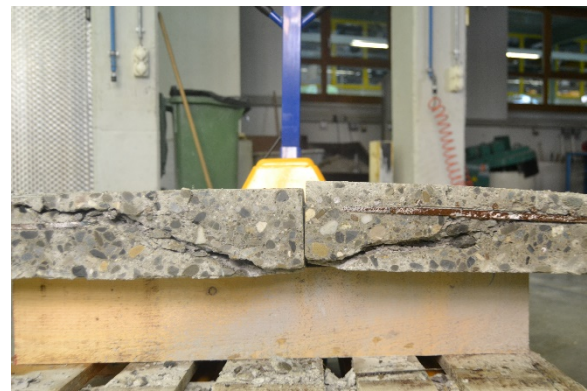
Figure 6 – Cracking pattern and internal shear crack of shear-reinforced slab BA01 after failure
