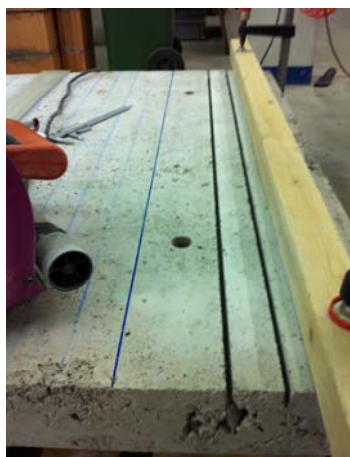
Figure 2 – BCN1 slots cutting
