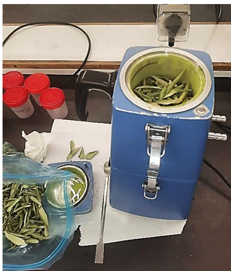
Figure 14: Freeze-dried leaves placed in the milling machine.
