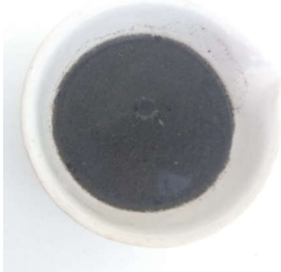
Figure 10. Sewage sludge used as inoculum.
