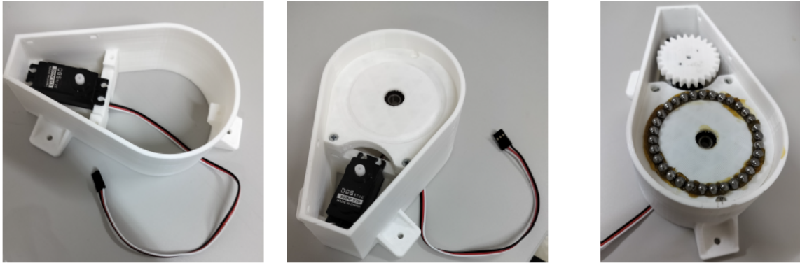
(a) Attaching the servo motor to the base support, enabling rotation. (b) Installing the main gear interacting with the base to spheres, drive rotation. (c) Adding the lower gear, and pulley to enable smooth base rotation.
