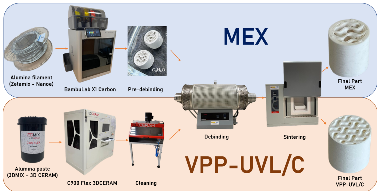
Figure 1 - Manufacturing stages for producing alumina parts using MEX and VPP-UVL.
