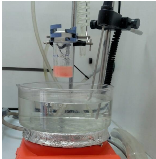
Figure 7. 4: Precipitation polymerization of the RAFT agent CPA.
