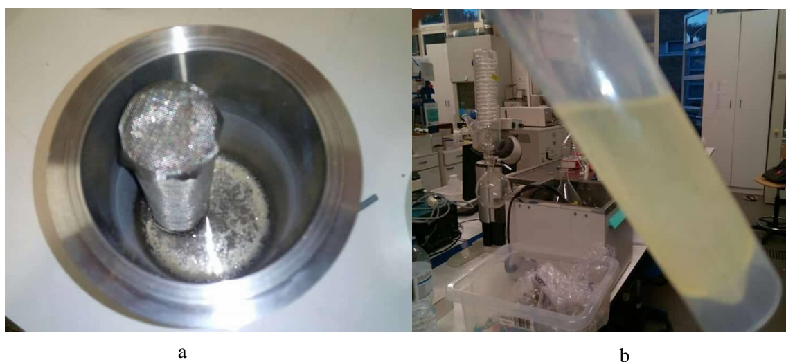
Figure 6.3: a) Basket containing the skin of chestnut fruit that was placed inside the extraction vessel used with supercritical CO 2 . b) Final yellow colored ethanolic solution obtained through the supercritical CO 2 extraction of the skin of the chestnut fruit.
