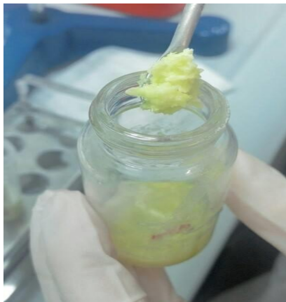
Figure 7.6: Precipitation polymerization performed presence of the RAFT agent CDTPA
