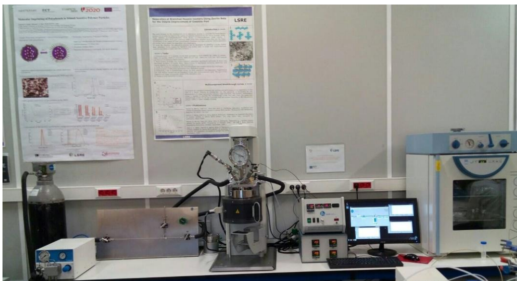
Figure 6.2: A view of the supercritical experimental unit used to obtain extracts from the skin of the chestnut fruit.
