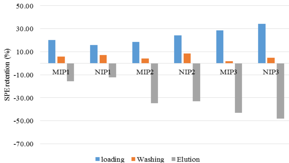
Figure 5.5: SPE adsorption of a mixture containing gallic acid + polydatin + resveratrol on the synthesized MIP and NIP materials. ACN/H 2 O 50/50 was used as first solvent.
