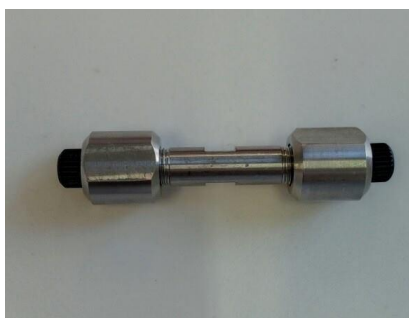
Figure 5.16: Packing columns used in experimental studies of the saturation and release polyphenols.
