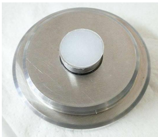
Figure 4.3: Final Aspect of the pellets for analysis Infrared Spectroscopy with Fourier Transform (FTIR).
