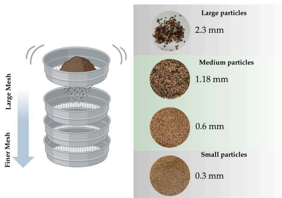
Figure 1. An overview of the particle size separation process, highlighting the corresponding mesh sizes utilised.
