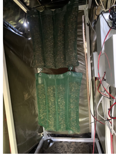
(b) Center – Acorn drying set-up; Right – datalogging and telemetry equipment.
