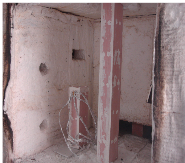
Fig. 2. Thermocouples, screws and position of the specimen inside the furnace.
