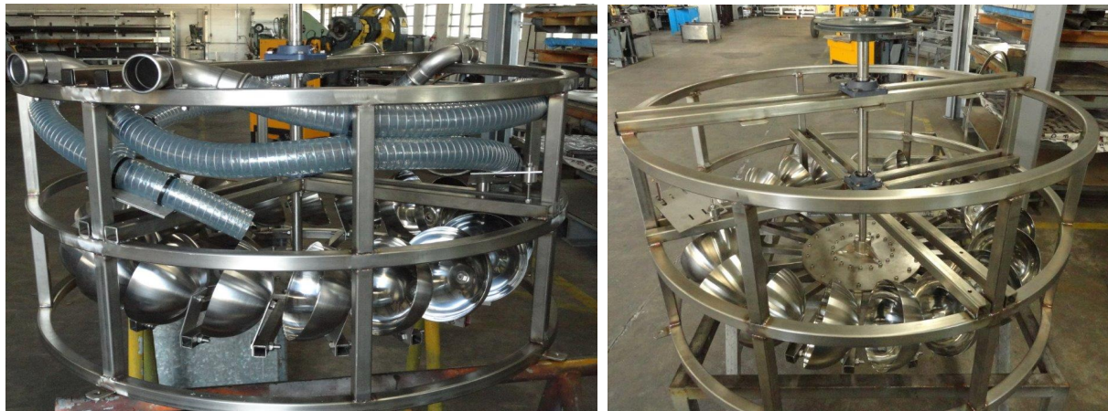
Figure 4.14: Water wheel under construction.
