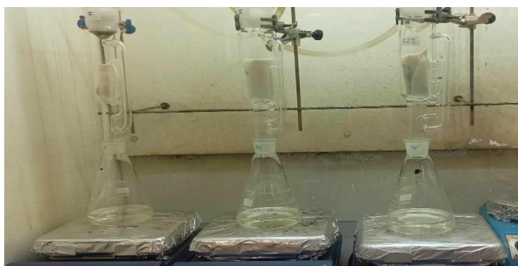
Figure 4. Soxhlet used for tocopherol extraction from walnut.
