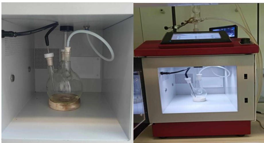
Figure 5. Microwave oven used for tocopherol extraction from walnut.
