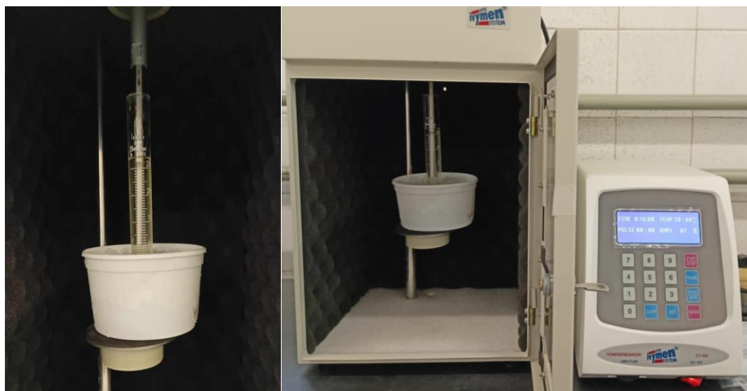
Figure 6. Ultrasound used for tocopherol extraction from walnut.
