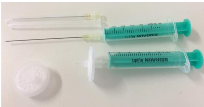
Figure 7. Syringes and filters used to collect the samples from the solutions.
