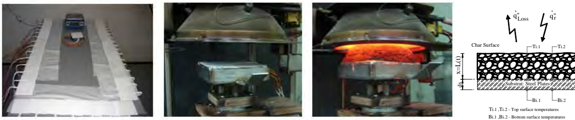
Fig. 1 – Coated steel plates, with fixed thermocouples, cone calorimeter setup and intumescence development.
