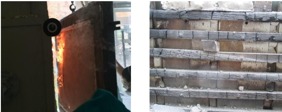
Figure 4: Final aspect of tabique panel
