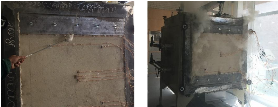
Figure 3: Integrity criteria proofing and smoke release
