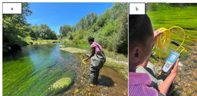
Figure 3.6. In situ evaluations of water quality in the River Tua. (Summer): a) measurement of water parameters using a multiparameter probe; b) results reading.
