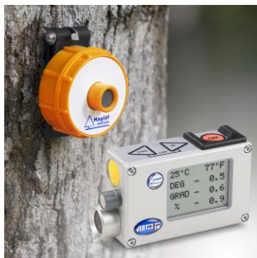
Figure 9: Hypsometer Vertex IV with transponder (Haglofcg, 2017)
