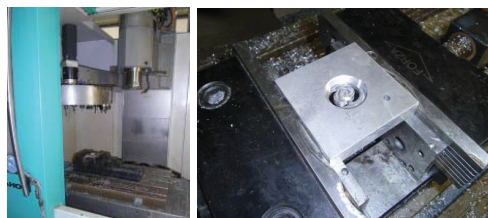
Fig. 4. The milling process: at left the CNC machine used to cut the pieces and, at right, an example of a machined assembly part.
