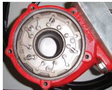
Fig. 2. Internal aspect of the “hot” part of a GT1749 variable-geometry turbocharger. Each of the eleven small levers controls a vane.
