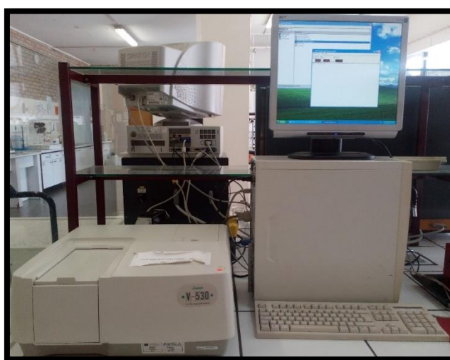
Figure 5.3 - UV Spectrophotometer system installed in the laboratory (LPQ).
