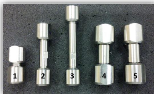
Figure 5.6 - Packing columns used in experimental studies of the saturation and release of drugs in polymers considering continuous operation mode.
