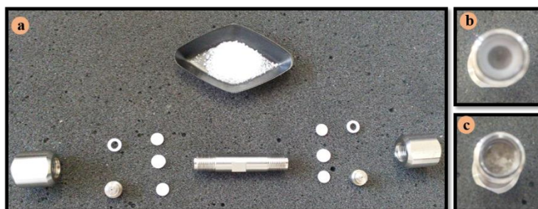
Figure 5.17 - Illustration of a column packing, a- elements of the column and polymer, b- column before packing, c- column after packing.
