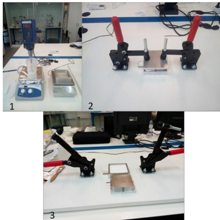
Fig. 1. Experimental set-up used for the ultralight microcellular PU synthesis at laboratorial scale: (1) reactive mixture stirring and heating; (2) mold lid fixation system, and (3) system opening and PU demolding.
