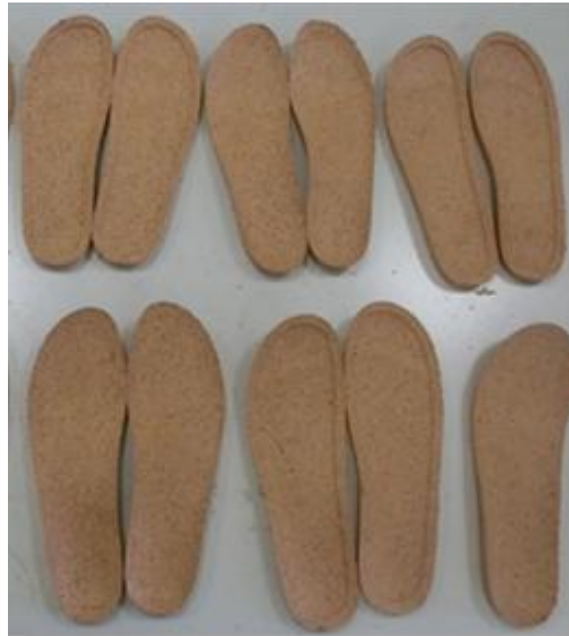
Fig. 2. Insoles samples produced by adding the grounded microcellular PU residues.
