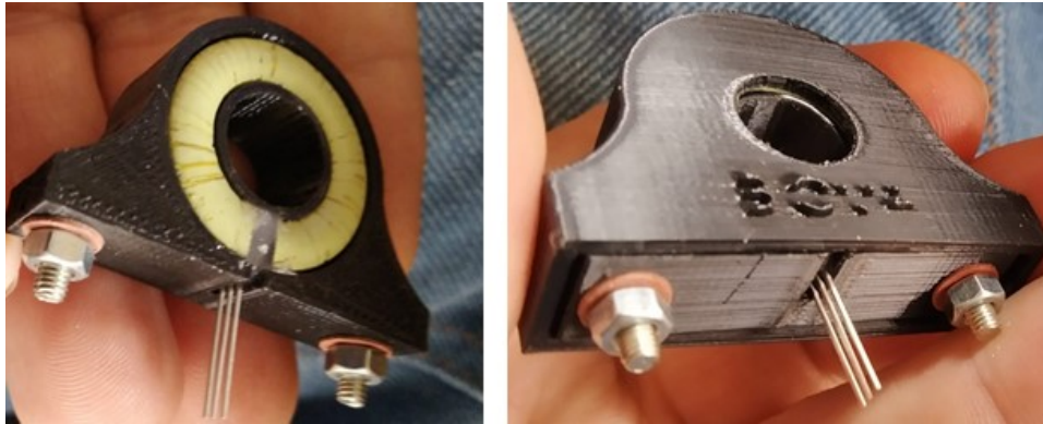
Figure 3.22: Final Result of Creating the Custom Current Sensor for BIOMA.
