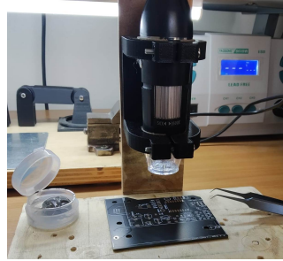
(b) Microscope used to help in soldering process.
