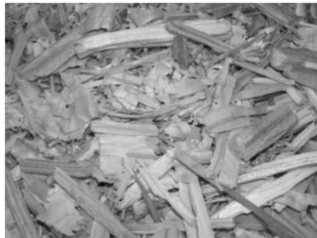
Figure 11 - Chips resulting from hammers chipper. Source: www.barkerdelivered.com
