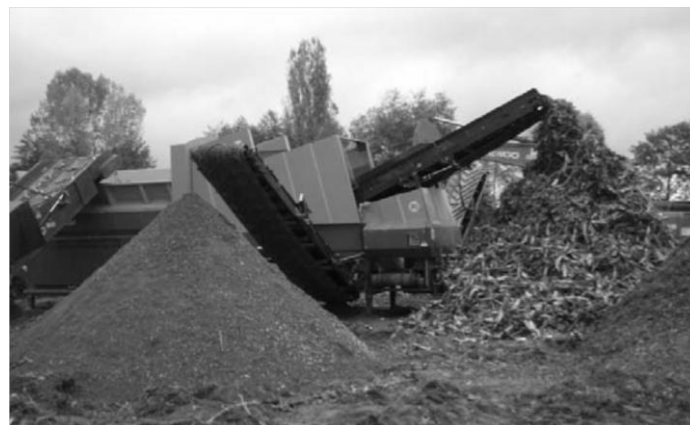
Figure 8 - Sieving wood chips produced from wood logs. The stack of chips (right) should pass new chipping to obtain better quality.
