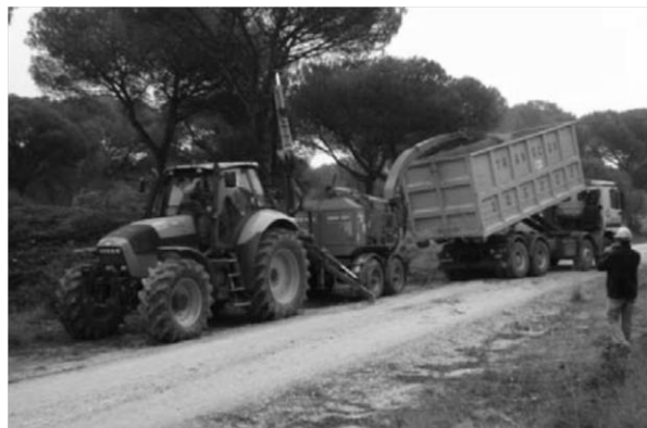
Figure 15 - FB being chipped near a forest stand and loaded directly into trailer.
