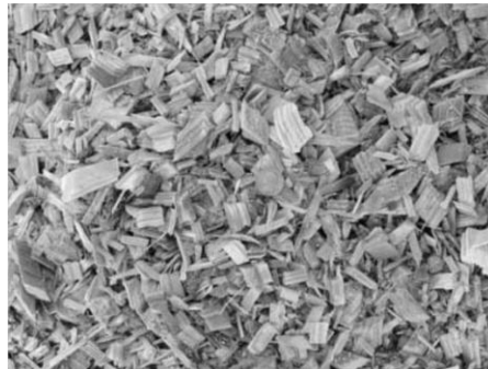
Figure 9 - Wood chips resulting from knives chipper. Source: www.barkerdelivered.com
