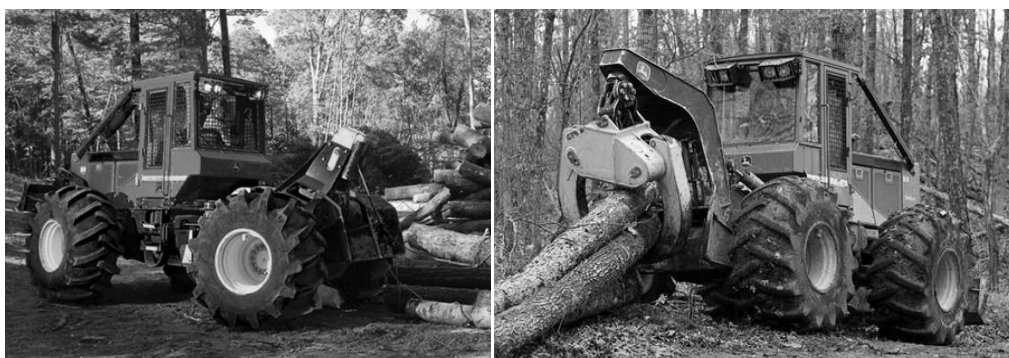
Figure 5 - Cable Skidder (left) and Grapple Skidder (right). Source: www.deere.com
