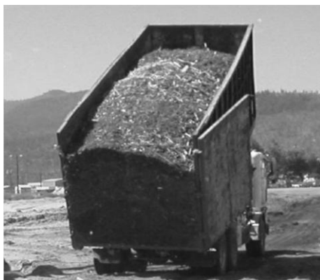
Figure 13 - Unloading wood chips using a hydraulic trailer. Source: (RE Consulting 2007)
