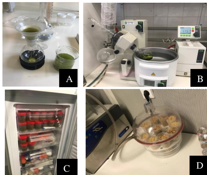
Figure 3-7 Sample preparation after the UAE: A. Filtration, B. Evaporation, C. Freezing, D. Lyophilization
