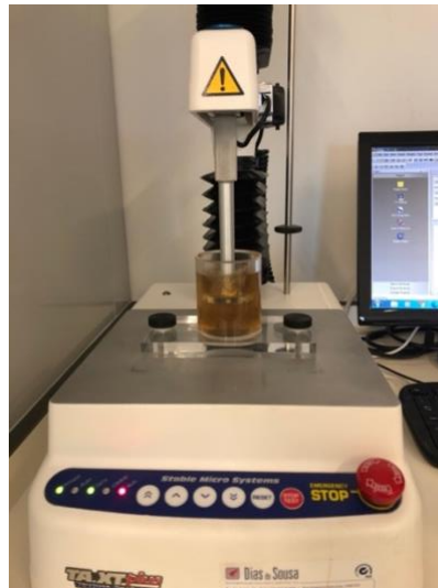
Figure 3-27 Stable Micro Systems' (Vienna Court, Godalming UK) TA.XT Plus
