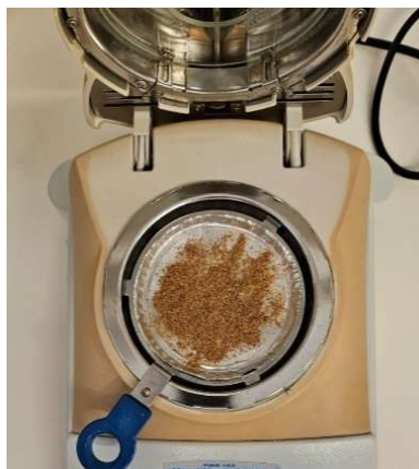
Figure 14 – Sample on the moisture analyzer Source - Own authorship (2025)
