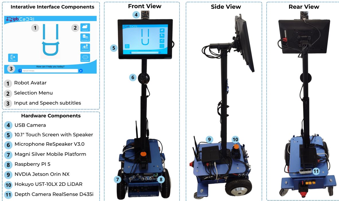
Figure 4.1: Preliminary version of the visitor guidance robot.
