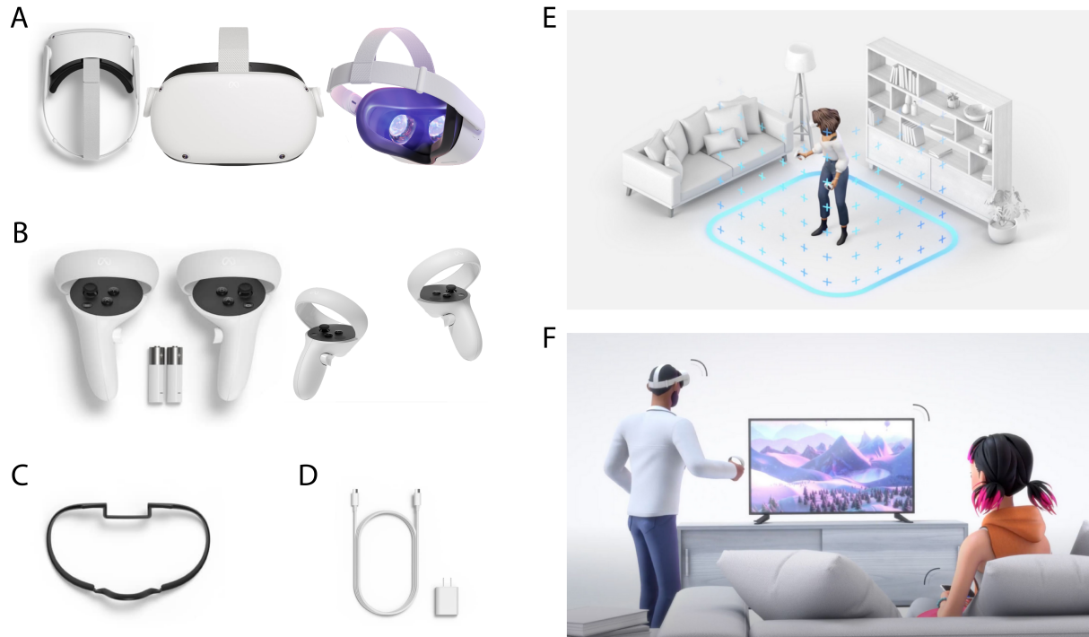
Figure 3.10: (A)VR headset (B)Controllers (C)Glasses spacer (D)Charger (E)Guardian (F)Casting.
