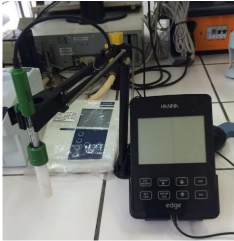
Figure 4. pH meter (Hanna Instruments)
