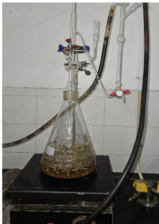
Figure 3. Essential oil extraction by Clevenger apparatus.
