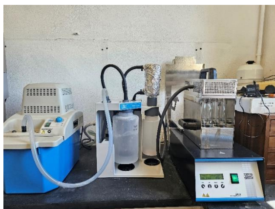
Figure 10. Kjeldahl digestion and distillation equipment.
