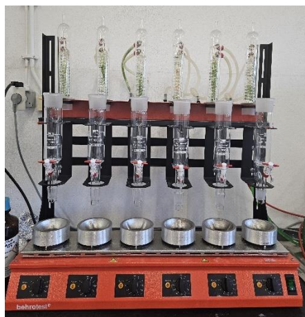
Figure 8. Soxhlet method equipment.
