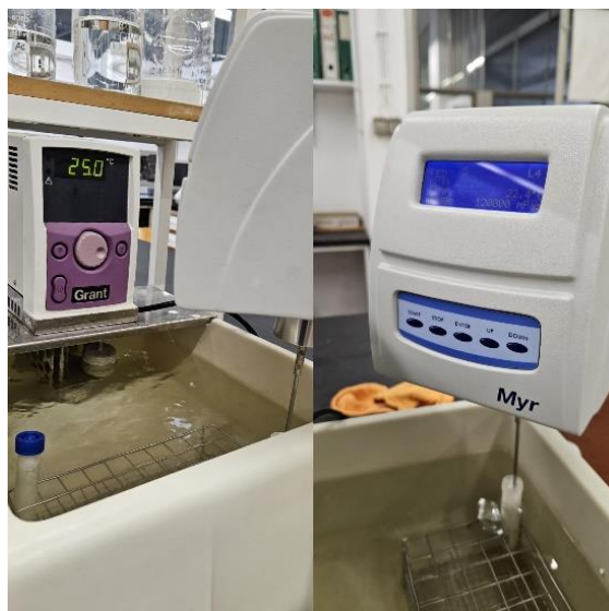
Figure 18. Viscosity measurement with the viscometer.
