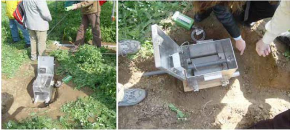
Figure 6. Runoff tipping-bucket recorder (Haute Normandie, France).
