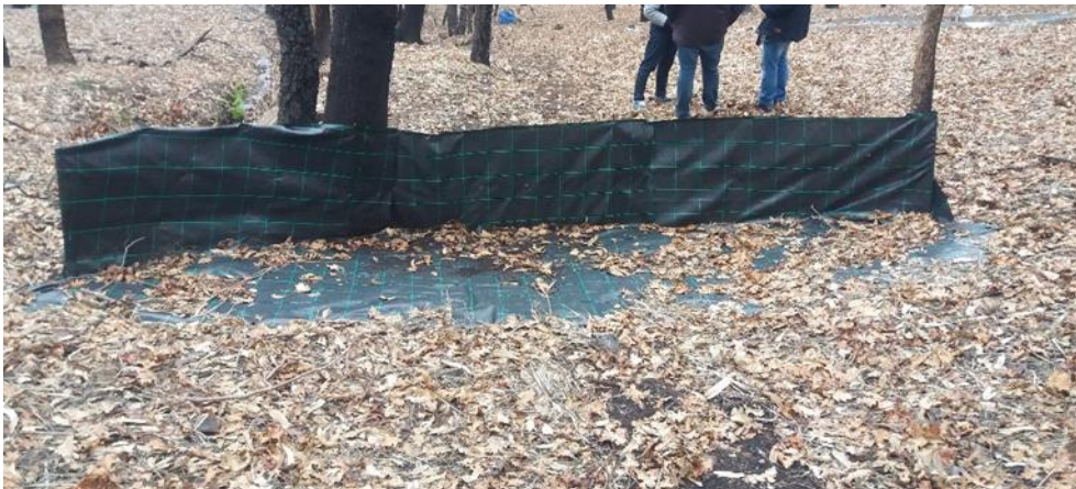
Figure 2. A silt fence (unbounded drainage area) installed in forest land, NW Portugal.
