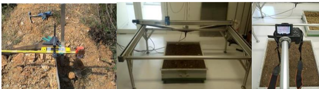
Figure 7. Assessing surface micro-relief with: home-made device on a micro-plot in NE Portugal (description in Fonseca, 2005) (left); laser profilemeter (centre) and camera capturing images for surface photogrammetric reconstruction (right) on soil samples in NW Spain (centre and right photos by Douglas Bandeira, description in Bandeira, 2019).
