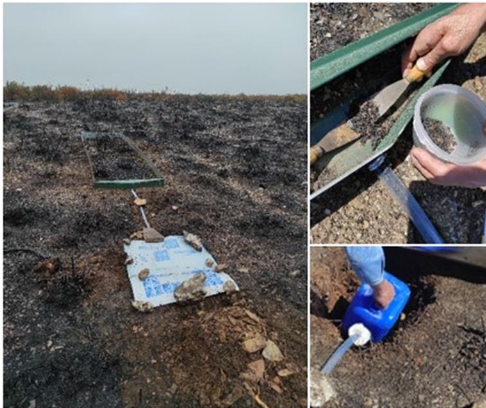
Figure 3. Erosion micro-plot (1 m wide, 4 m long) installed in a burnt area at Aveleda, NE Portugal (left), with collection of washed soil particles and ashes (top right), and runoff water and suspended sediment (bottom right) (study area described in Fonseca et al, 2017).
