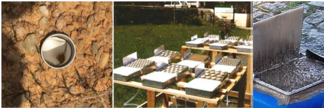
Figure 1. Splash cup, 5.5 cm diameter installed in a field experiment (Fonseca, 2005; Figueiredo et al. , 2012) (left), splash boards installed in outdoor micro-plot experiment with simulated rock fragments (Figueiredo and Poesen, 1998) (centre), and board capturing splashed particles during a rainfall simulation micro-plot experiment using burnt soil samples (Alves, 2018 and Royer, 2019) (right).
