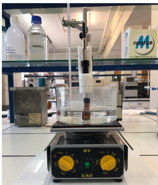
Figure 4. SPME extraction using a manual holder, agitation and heating plate with a thermometer for temperature control and 4 mL amber vials.
