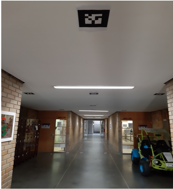
Figure 5.8: Fiducial markers fixed on the ceiling of the hallways in the robotics laboratories area.
