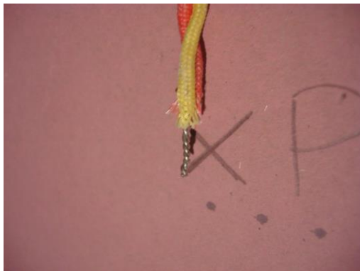
Twisted thermocouple on gypsum board
