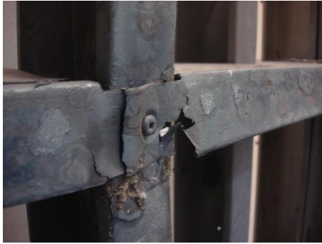
Brittle fracturing behaviour of the steel
