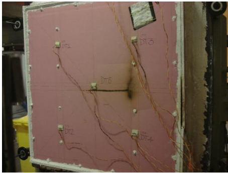
Unexposed surface after fire exposure
