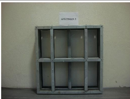
Steel frame condition after the test
