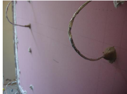
Bed thermocouple on gypsum board (twisted tip)
