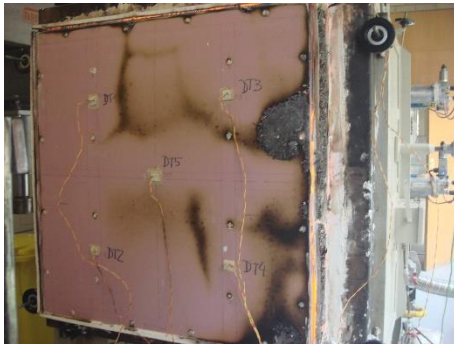
Unexposed surface after fire exposure
