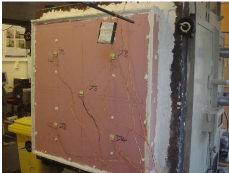
Unexposed surface after fire exposure
