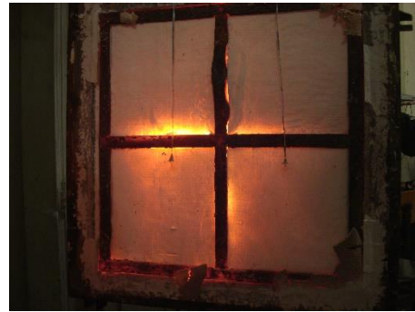
Exposed side after fire exposure
