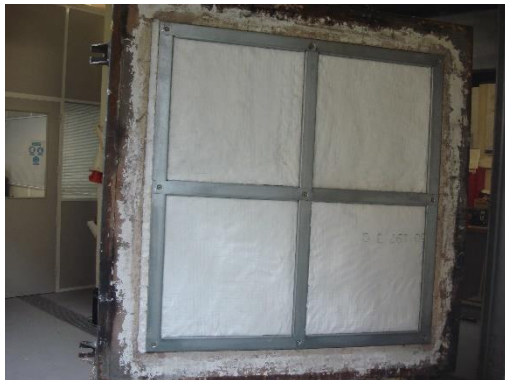
Framework insulated with ceramic fibre
