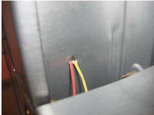
Welded thermocouple on steel stud
