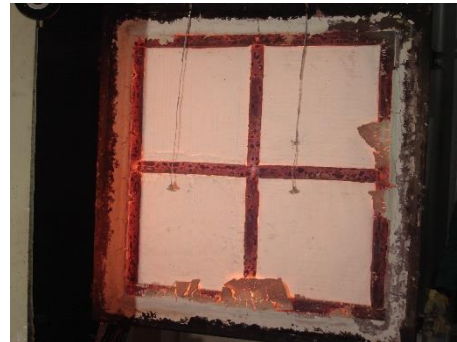
Exposed side after fire exposure
