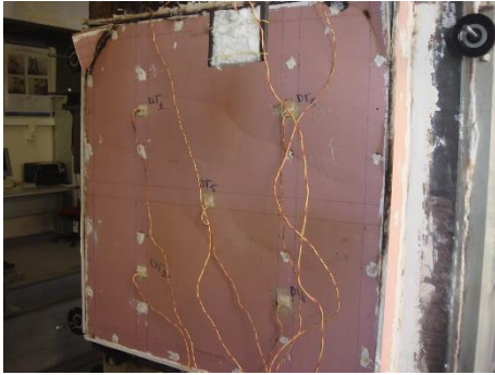
Unexposed surface after fire exposure
