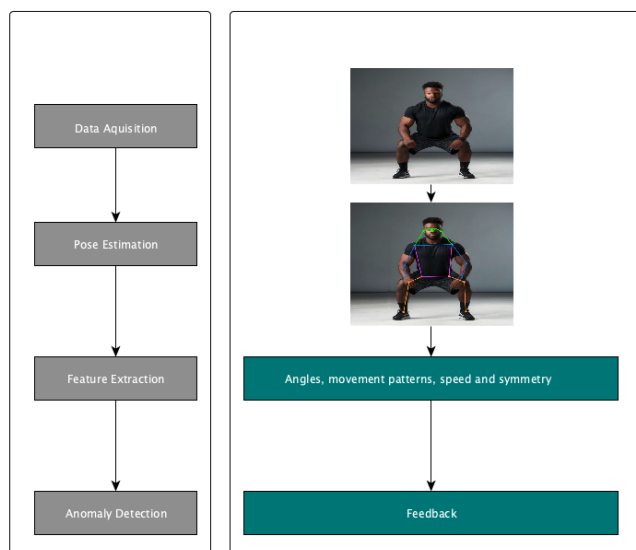
Fig. 1. System pipeline for the mobile rehabilitation app, showing the stages from video input and pose estimation to feature extraction, anomaly detection, and real-time feedback based on movement patterns, speed, angles, and symmetry.
