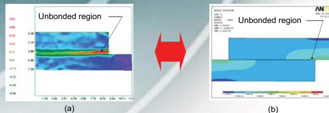
Figure 2 . Detection of unbonded region: (a) experimental; (b) numerical.
