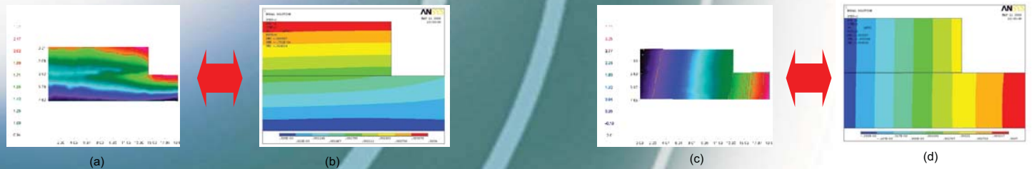
Figure 1. Displacement field: u direction - (a) experimental results and (b) numerical simulation ; v direction - (c) experimental results and (d) numerical simulation .
