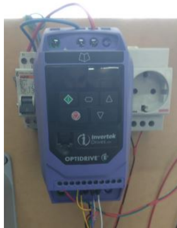
Figure 4.5: SFC used in the tests: Invertek Optidrive E3 1HP Single-Phase Input/Output.
