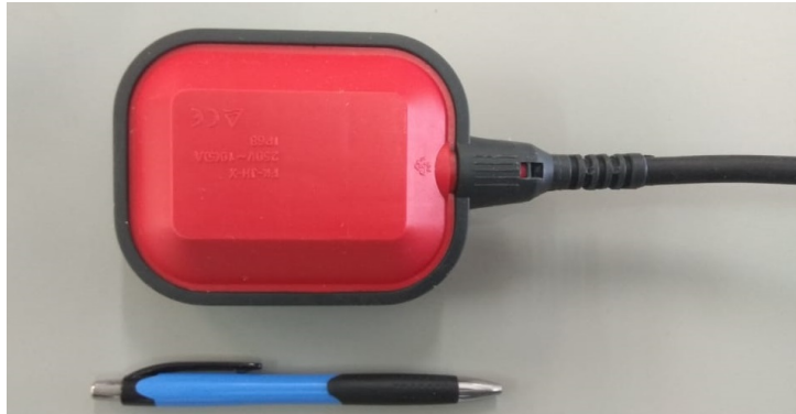
Figure 3.27: Exemple of a electrical buoy.
