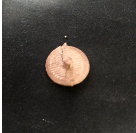
Figure 5.1: Fissure on Cellulose electrode breaking the thin film
