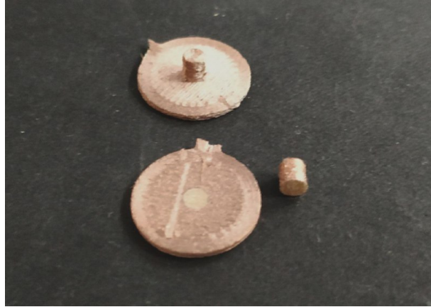
Figure 3.5: Cellulose electrode with its connector broken after several cycles of connecting and disconnecting
