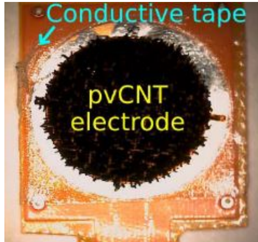
Figure 2.3: Patterned Vertical Carbon Nanotubes electrode fixed on conductive tape. Imagem from [39]
