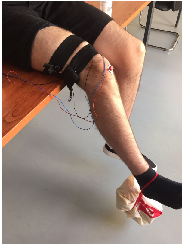
Figure 4.4: Acquisition with electrodes fixed by elastic bands while using weight to force the muscle
