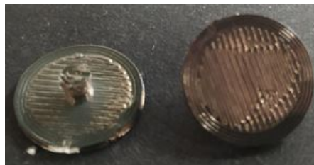
Figure 5.4: TiN electrode without apparent damages after 3 days immersed in artificial sweat
