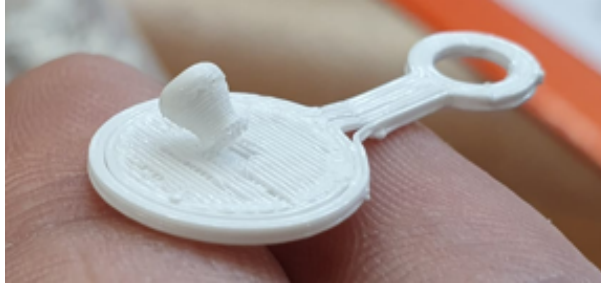
Figure 3.7: PLA snap button connector broken after disconnection
