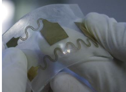
Figure 2.5: PDMS with gold serpentine patterned electrode. Example from [48]
