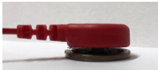
Figure 3.12: Last snap button version connected to the female snap connector
